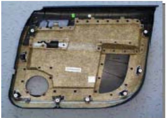
Figure 6: Automotive door-inliner made from jute, flax, hemp, sisal fiber reinforced composites
