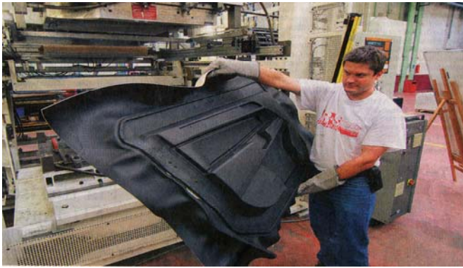
Figure 6: Automotive door-inliner made from jute, flax, hemp, sisal fiber reinforced composites
