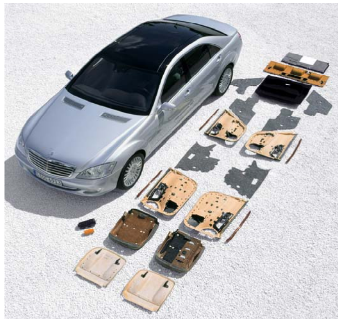
Figure 10: Newest Mercedes S class automotive components made from different bio fiber reinforced composites
